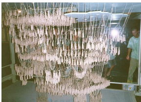
Colònia Güell model Hanging and inverted images of a Gaudi design.
