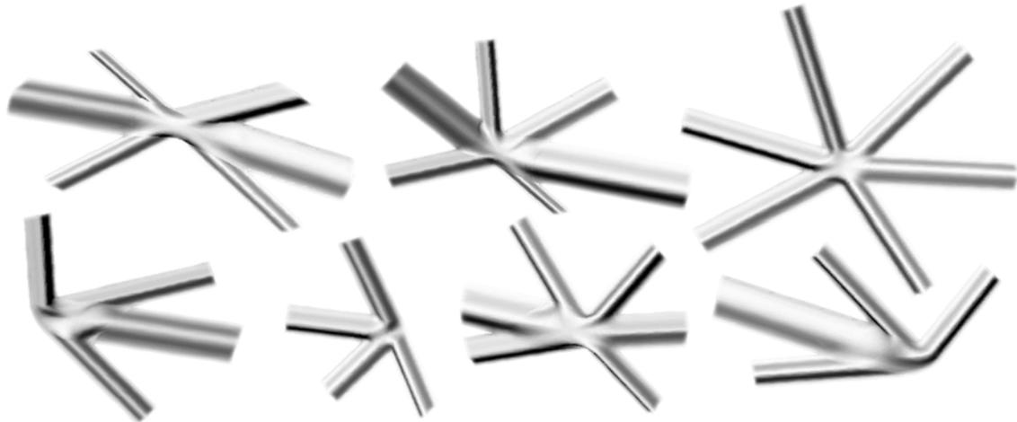
**Figure 6. Joint studies from a previous project for intersections of members of unequal diameter in different spatial configurations using a parametric representation**
