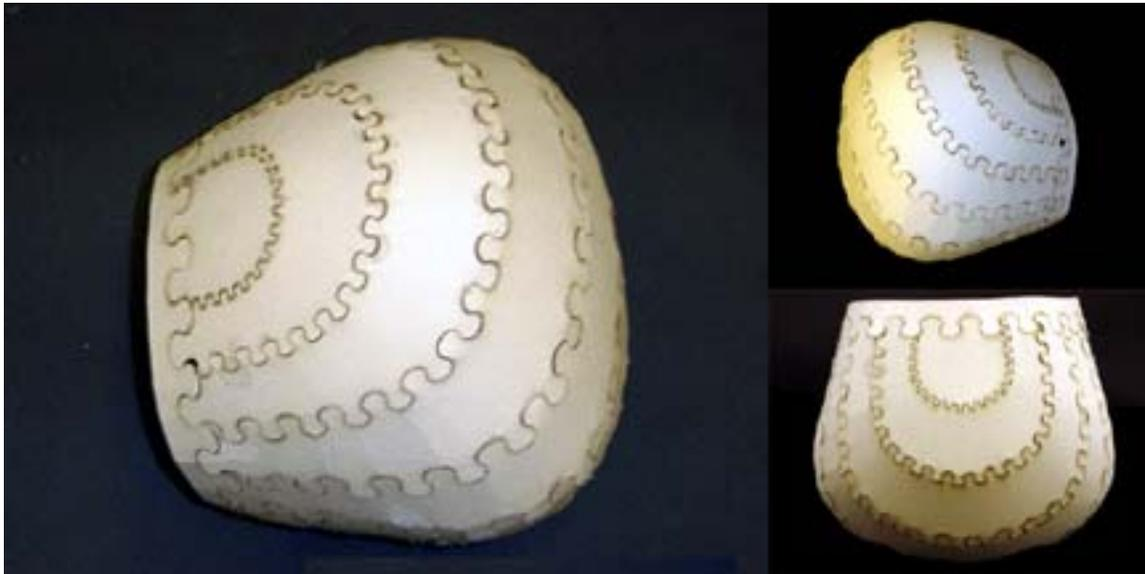
Figure 1. Example of puzzle joint surface
